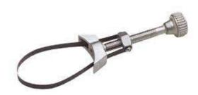
Easy removal of oil filters by tightening the metal strip around the filter with the screw mećhanism
